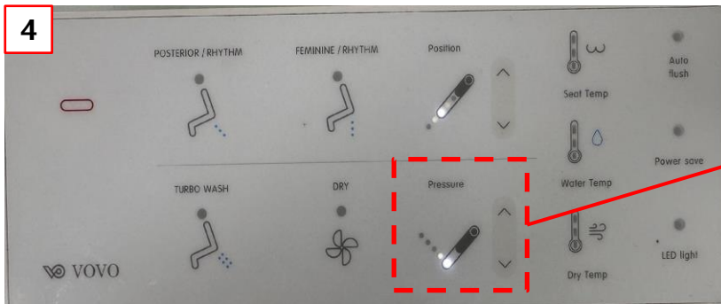
④ Check the water pressure setting on the remote and set it to level 5.
