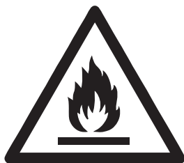
caution, risk of fire
