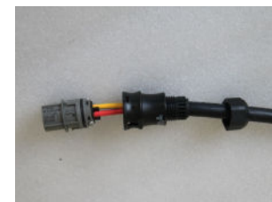
▲ Figure 4.16 Connect Wires to the Terminal
