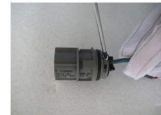
▲ Figure 4.16 Connect Wires to the Terminal
