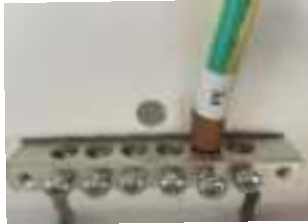
Figure 4.10 Grounding Terminal on Heat-Sink
