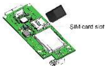
Figure 9: Inserting the card into the GSM modem
