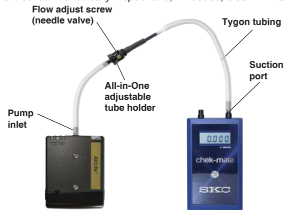
Calibration train with All-in-One connected to pump
