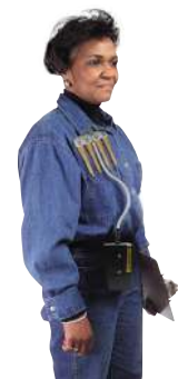
Clip tube holder to worker and pump to belt.
