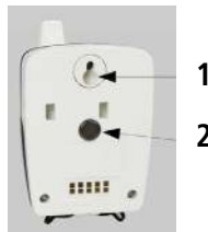
1. Wallmount and lace eyelet 2. Magnetic mounting
