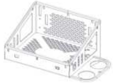
BEVERAGE COOLER HOLDER (with Trim Lok); P/N: 8SV-WA-00372 (QTY.: ONE)
