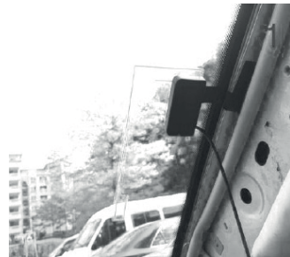
Stick the transparent part of the antenna on the windshield and put the black part on the metal frame.
