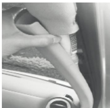
Remove the cover of the A-post
