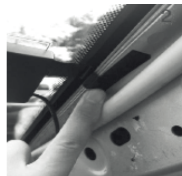
Stick the transparent part of the antenna on the windshield and put the black part on the metal frame.
