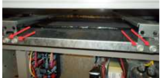
FIGURE 6 Remove Four Screws
